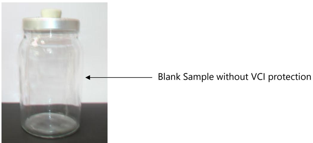
The four test sets were stored for a period of  $(20 \pm 0.5)$  hours at a room temperature. At the end of the storage period, the jar covers were removed from the test jars, the freshly
